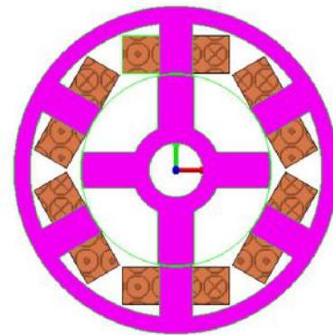
Fig. 8. Model of the VR stepping motor under MagNet Infolytica.
