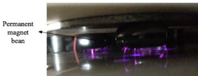
Figure 6. The arrangement of small permanent magnets on the high voltage electrode.
