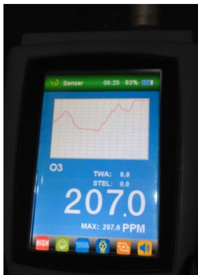
Figure 11. Ozone measurement with a gas analyzer.
